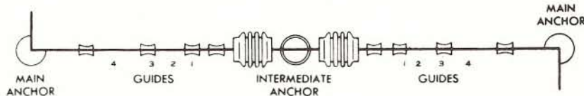
DIAGRAM #2 Two Expansion Joints in longer pipe run than that shown in Diagram #1. Intermediate anchor between main anchors forms individual expanding and contracting sections. Expansion Joints are installed between intermediate and main anchors.
